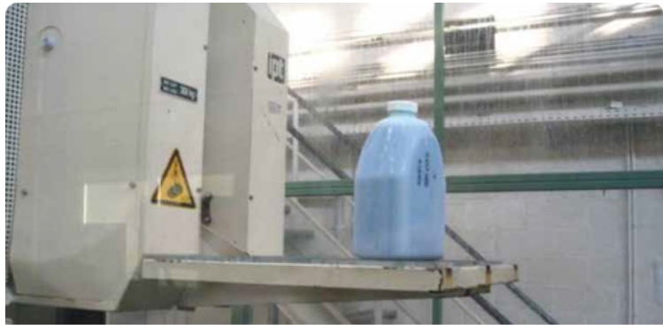
Figure 1: Drop test set-up
