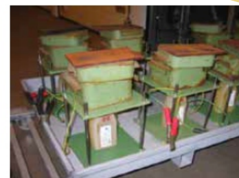
Figure 4: Diesel stacking test set-up
